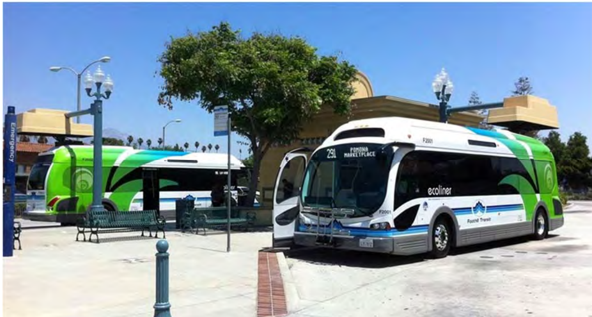
Figure 1-10. Proterra electric buses operated by Foothill Transit, charging at the overhead charging stations in the Pomona Transit Center (photo, courtesy of Proterra)
