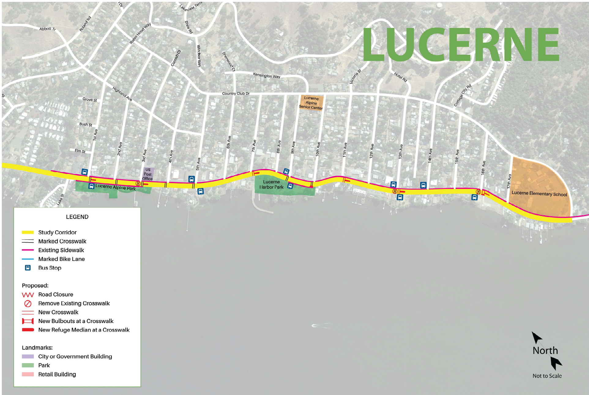
SR 20 Northshore Communities Traffic Calming Plan and Engineered Feasibility Study Figure 9 – Proposed Crosswalk Improvements (Lucerne)
