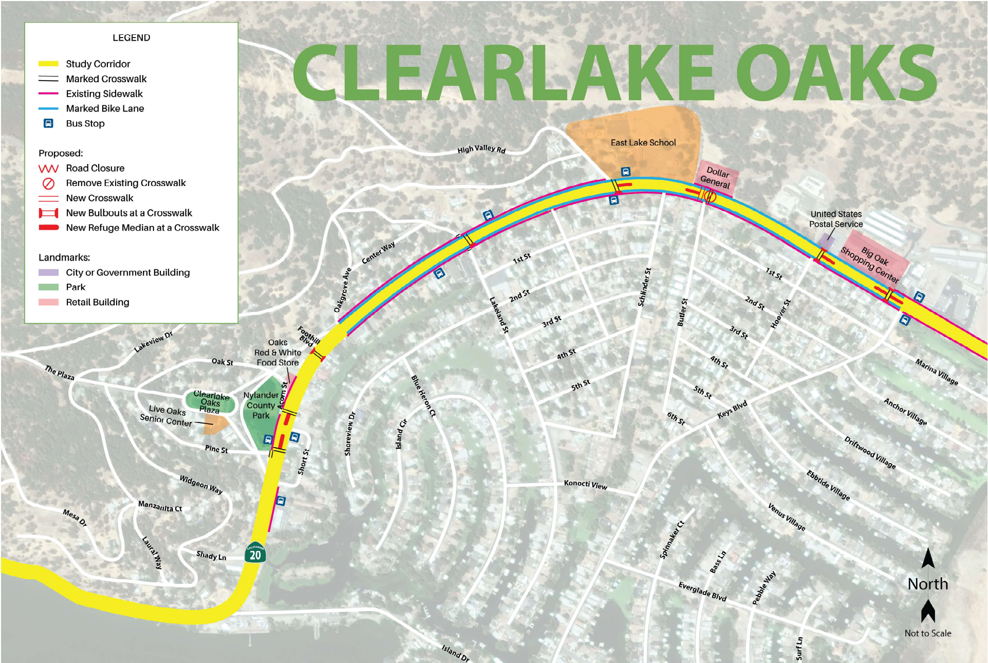
SR 20 Northshore Communities Traffic Calming Plan and Engineered Feasibility Study Figure 10 – Proposed Crosswalk Improvements (Clearlake Oaks)
