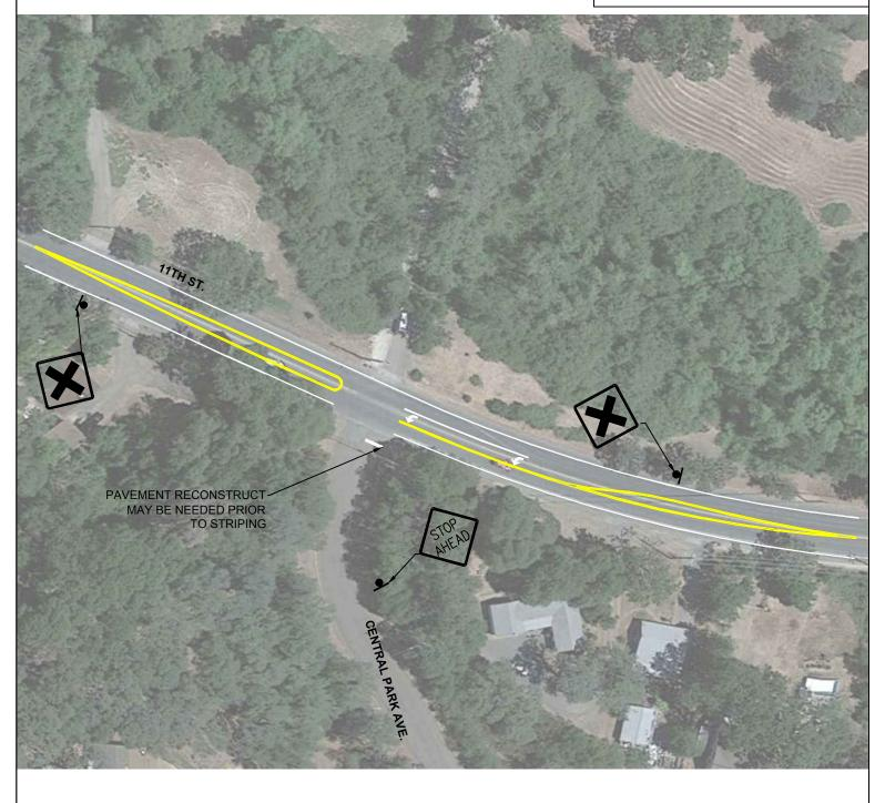
NOTE: INTERSECTION WARNING SIGNS AND STOP AHEAD SIGN TO BE PLACED A MIN. 200' AND 100' FROM THE INTERSECTION, RESPECTIVELY. ADDING LEFT TURN POCKET MAY REQUIRE BIKE LANES TO BE REMOVED TO MAINTAIN APPROPRIATE LANE WIDTHS. THIS IS A PRELIMINARY CONFIGURATION AND FIELD VERIFICATION OF ROADWAY WIDTH SHALL BE VERIFIED PRIOR TO THE CREATION OF CONSTRUCTION DOCUMENTS.
