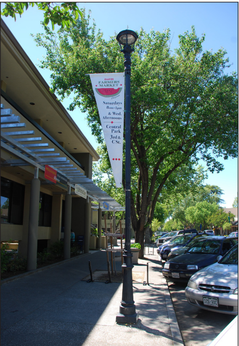
Top: Pedestrian scale lights oriented to the sidewalk versus automobile-scale light. Bottom Left and Right: examples of traditional street-light poles with modern energy-efficient fixtures that aim illumination toward the ground and reduce glare that obscures night sky visibility. The lampposts are also equipped for wayfinding and thematic signage.
