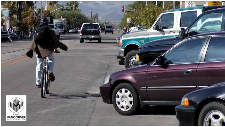
The photo shows how back-in angled parking can improve the visibility of passing bicyclists to motorists.
