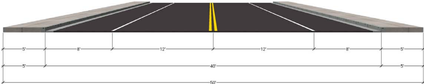
Above: the cross section above illustrates typical conditions with a sidewalk on both sides of the street.
