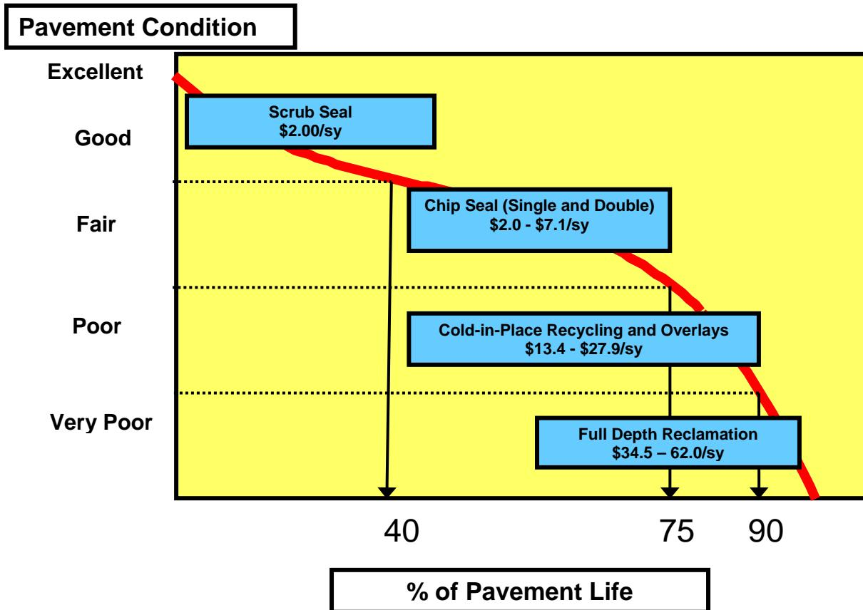
**FIGURE 3. Costs of Maintaining Pavements Over Time**
