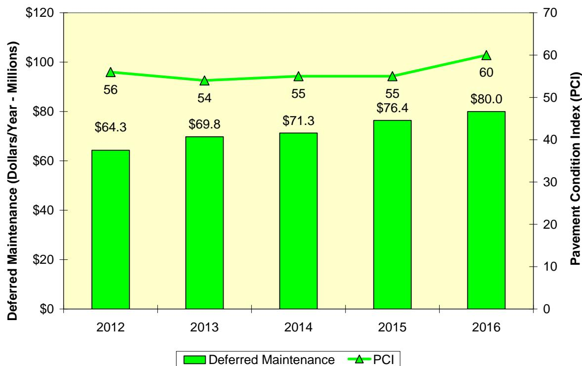
**FIGURE 6 PCI vs. Deferred Maintenance for \$6.0 Million Per Year**
