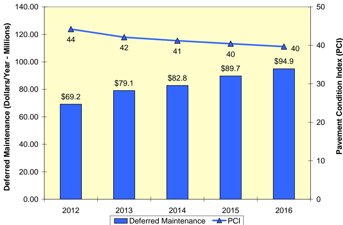
**FIGURE 4. PCI vs. Deferred Maintenance for \$1,100,000 Per Year**
