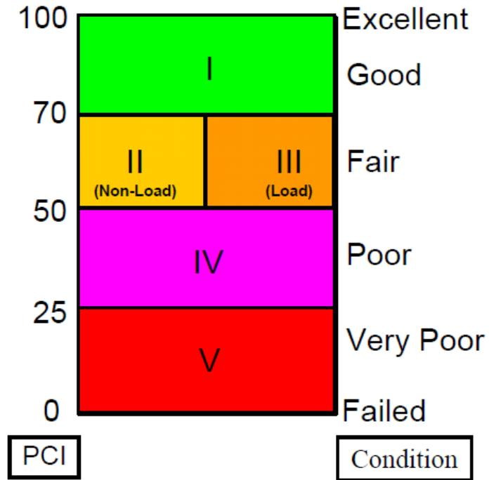
**FIGURE 1. Pavement Condition Categories by PCI**
