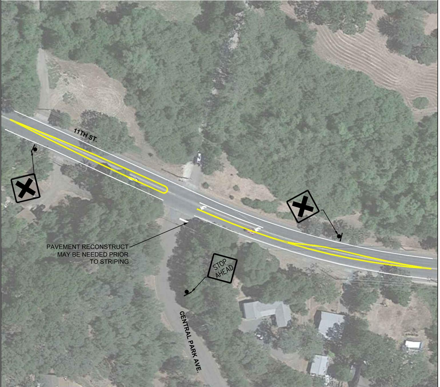
NOTE: INTERSECTION WARNING SIGNS AND STOP AHEAD SIGN TO BE PLACED A MIN. 200' AND 100' FROM THE INTERSECTION, RESPECTIVELY. ADDING LEFT TURN POCKET MAY REQUIRE BIKE LANES TO BE REMOVED TO MAINTAIN APPROPRIATE LANE WIDTHS. THIS IS A PRELIMINARY CONFIGURATION AND FIELD VERIFICATION OF ROADWAY WIDTH SHALL BE VERIFIED PRIOR TO THE CREATION OF CONSTRUCTION DOCUMENTS.
