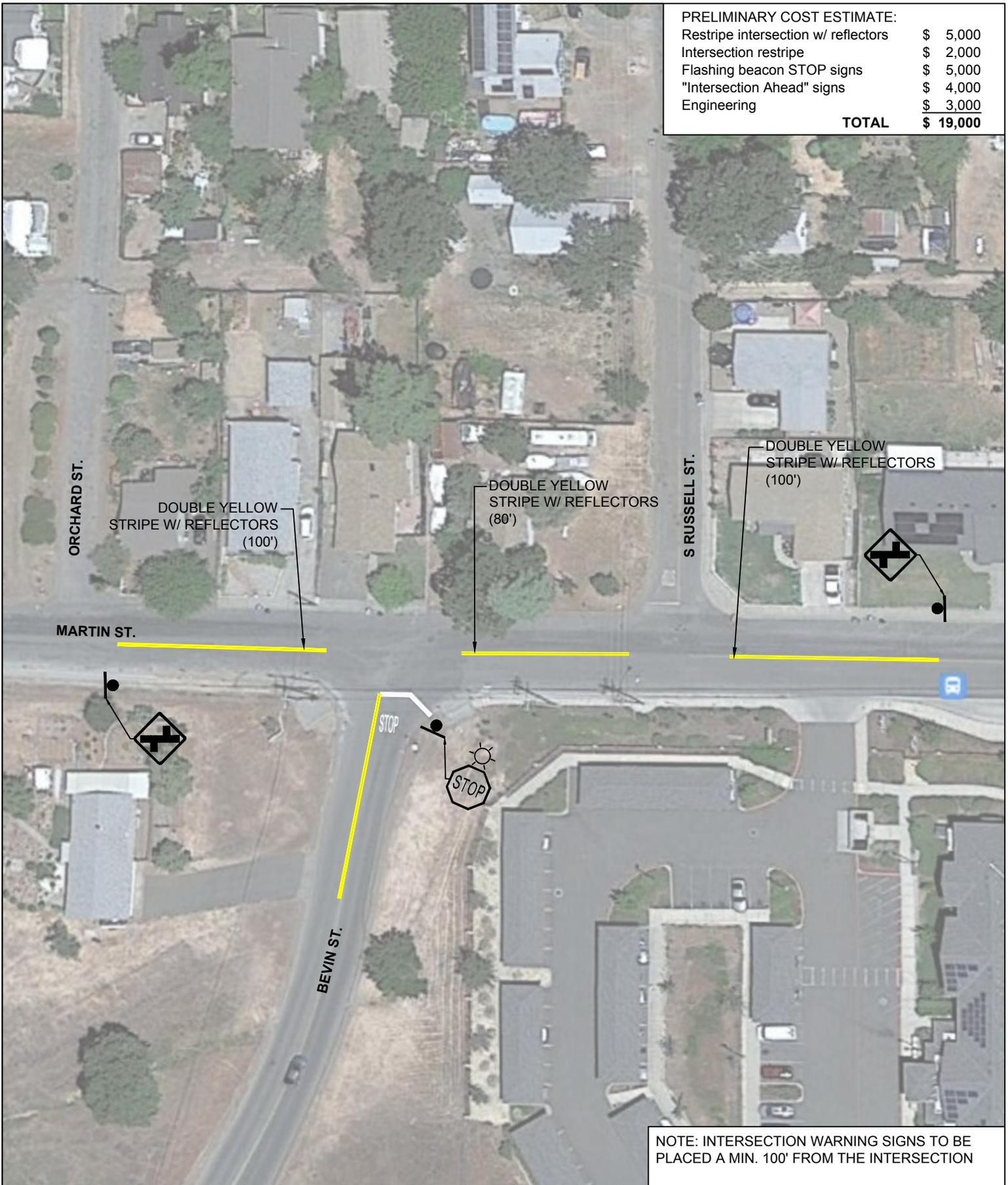
NOTE: INTERSECTION WARNING SIGNS TO BE PLACED A MIN. 100' FROM THE INTERSECTION
