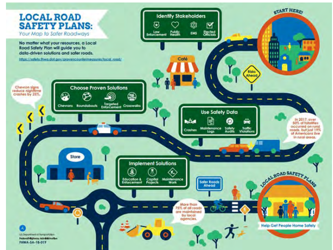
Exhibit 1. The LRSP Process – Identify Stakeholders, Use Safety Data, Choose Proven Solutions, and Implement Solutions. Source: FHWA
